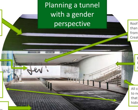
Roof extends no further than to have overview from both sides of tunnel: Create overview
